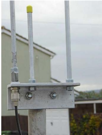
(Note: When cutting the threads, make sure they are perfectly square, else you will end up with an antenna that looks a bit strange with elements leaning at odd angles. Also, aluminium will tend to grab the tap or die so a little lubricant will help give you a clean thread, but make sure you clean it thoroughly before final assembly.)
